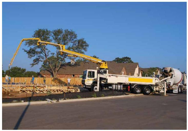
Boom position sensors and two axis level sensors help improve pumper productivity through automated home/stow positioning and auto leveling. Cylinder end-of-stroke dampening helps reduce boom fatigue and shortens boom placement time through smoother operation.
